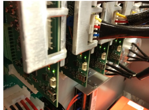
LED indicators on amplifier units
