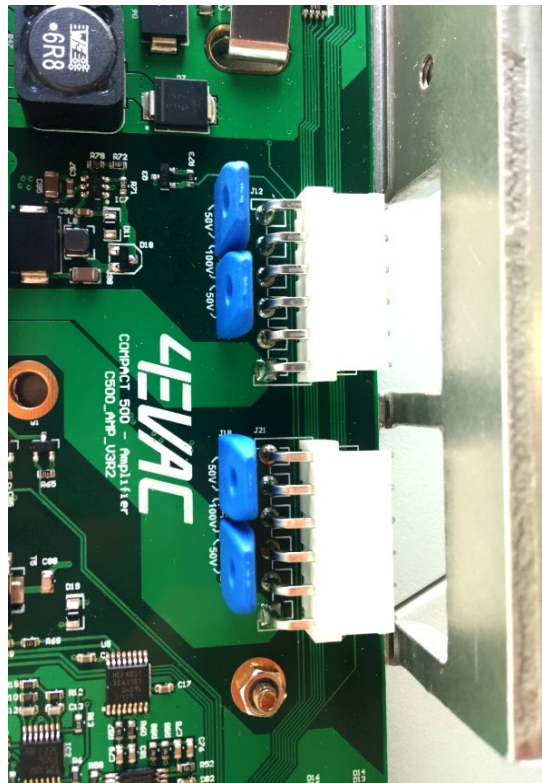
Jumper setting 50V per channel – amplifier unit
