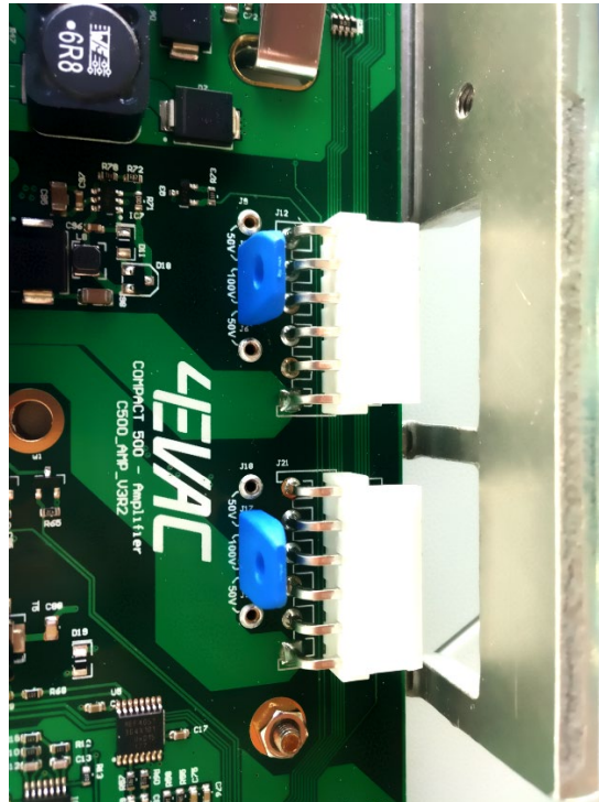
Jumper setting 100V per channel – amplifier unit
